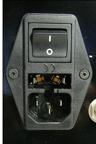
FUSE HOLDER REMOVED
