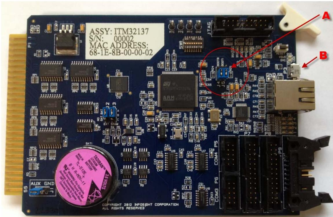
Figure 1 – Location of Boot Mode Jumpers “A” and Micro USB Connector “B”
