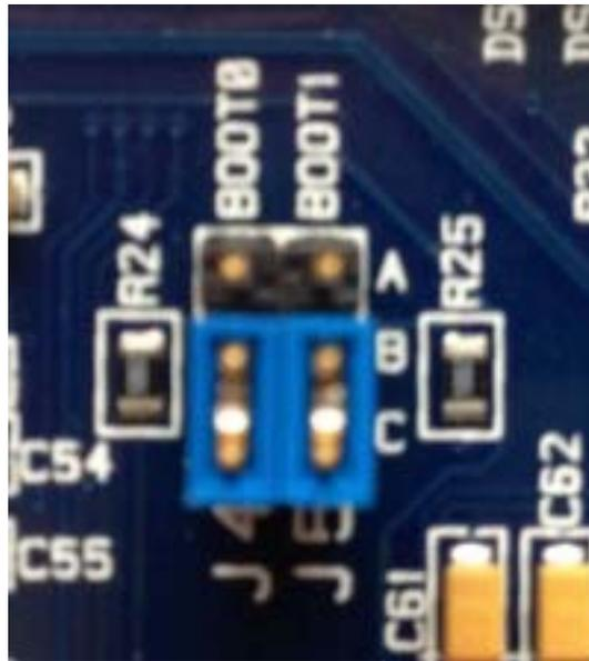
Figure 10 – Jumpers in Run Position
