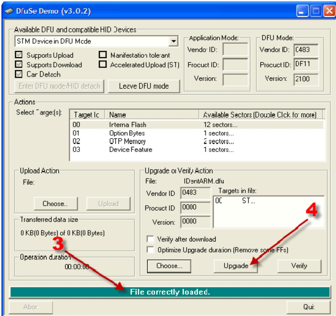
Figure 7 – File Loaded and Ready to Upgrade
