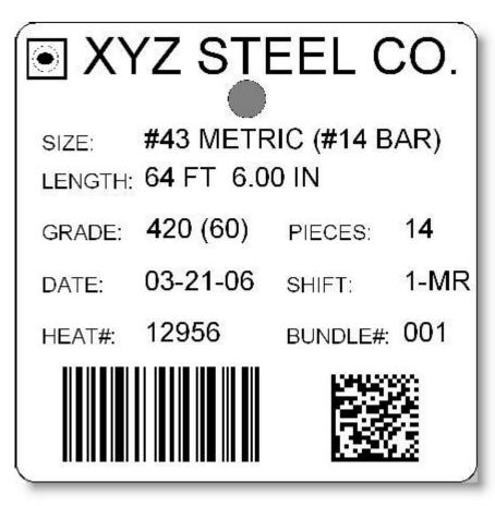
As you can see, this label has several text fields including fields that contain data that changes on each tag, as well as label fields that are fixed (do not change) and serve to describe the associated data fields. There are two barcodes on this label, one that is a 1D code that contains a small amount of data, and one that is a 2D code that contains more information than can fit in a standard 1D code. Finally, a company logo appears to identify your organization.
