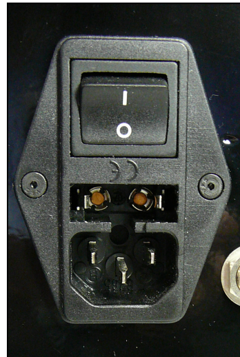
FUSE HOLDER REMOVED
