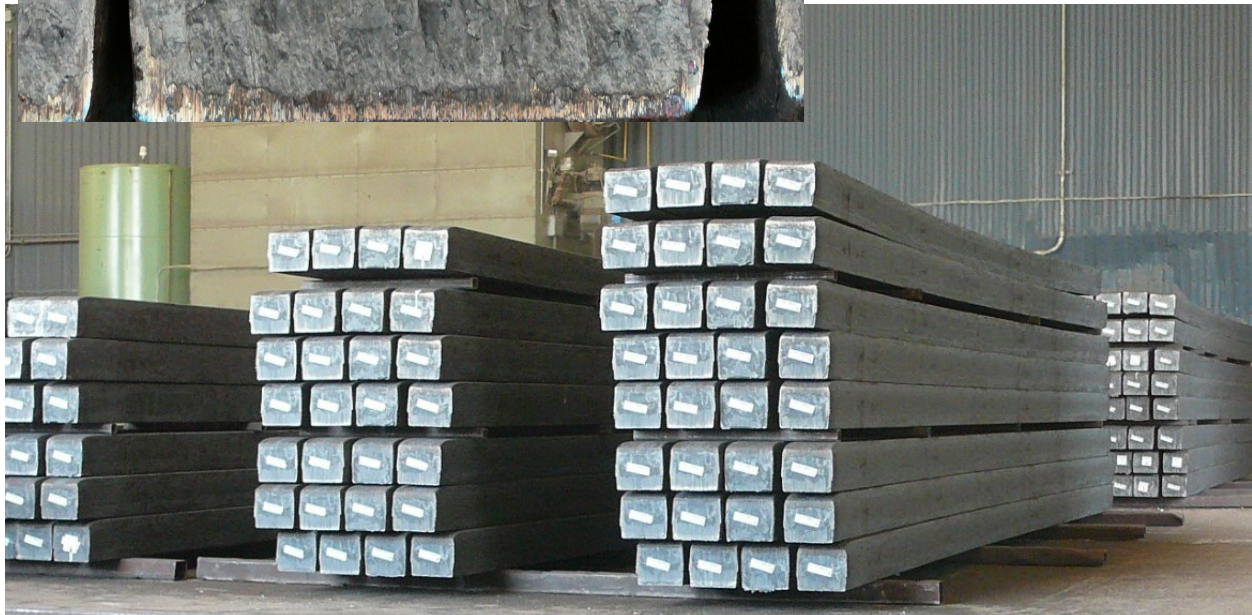
Below—stacks of bars with nailed-on tag ID
