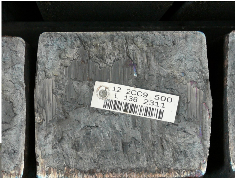
Below—stacks of bars with nailed-on tag ID
