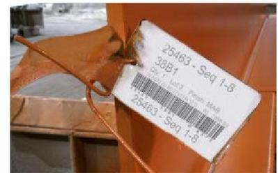
This metal bar code tag was sent through blast cleaning and painting. After painting, the tag's clear protective laminate cover was removed, revealing the bar code and part number underneath.
