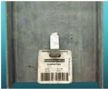
This isn't a paper tag, but a metal tag with a white coating. The tag remained on the girder throughout the hot-dipped galvanizing process.
