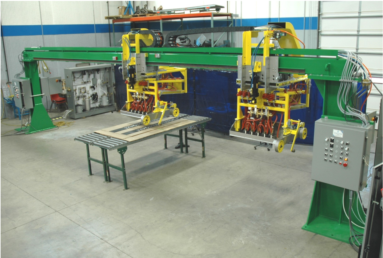
5-head I-DENT® Hot Plate marker with dual carriages— shown in the InfoSight shop
